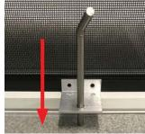
**Locking bracket (interior install)** - Placement: screens 24" and smaller (1 bracket supplied) are center installed. Screens 24" and larger (2 or 3 brackets supplied) are installed 6" from each end, and if 3rd bracket provided install in the center. Fasten aluminum locking bracket to bottom of screens and drill hole (5/16" dia. x 1/2" deep) into sill to slide pin down into.
