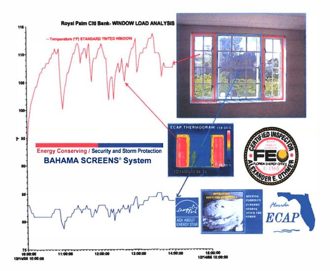
The center window had been retrofitted with the **BAHAMA SCREENS**. The *THERMOGRAM (Infrared heat image)* clearly shows the reduced heat loads (blue areas) being produced by the **BAHAMA SCREENS** in comparison to the standard windows on each side of it that have window tint applied to them (red areas).
