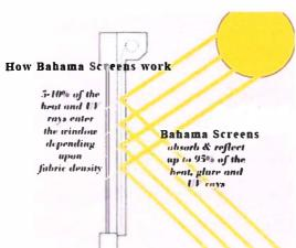
Exterior Bahama Screens block up to 95% of the heat, glare, and ultraviolet rays, without blocking the view. Mounting Exterior Solar Screen Shades on the outside of the window blocks the sun's heat before it enters the glass, instead of trying to reflect unwanted heat back out.
